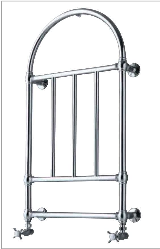
■ SSARC1 • Radiatore a muro ad arco con griglia mm.990x530 DT60° 422 Kcal/h - 481 Watt Radiateur mural arc avec grille mm.990x530 DT60° 422 Kcal/h - 481 Watt Wall mounted arch radiator with grid mm.990x530 DT60° 422 Kcal/h - 481 Watt
