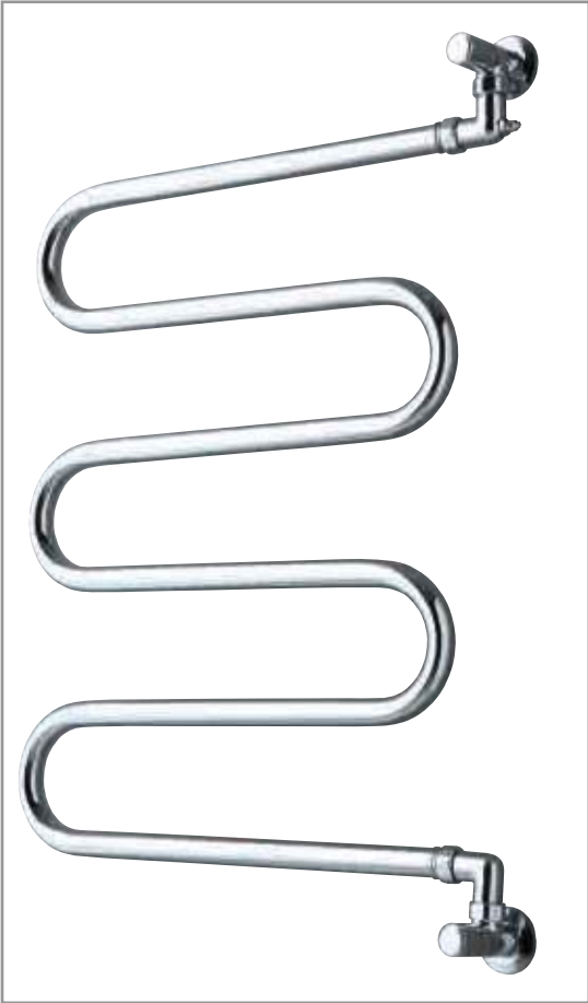
■ SSERP6 • Radiatore a muro serpentina 6 barre mm.785x530 DT60° 160 Kcal/h - 185 Watt Radiateur mural serpentin 6 barres mm.785x530 DT60° 160 Kcal/h - 185 Watt Wall mounted radiator with 6 rails mm.760x650 DT60° 160 Kcal/h - 185 Watt
