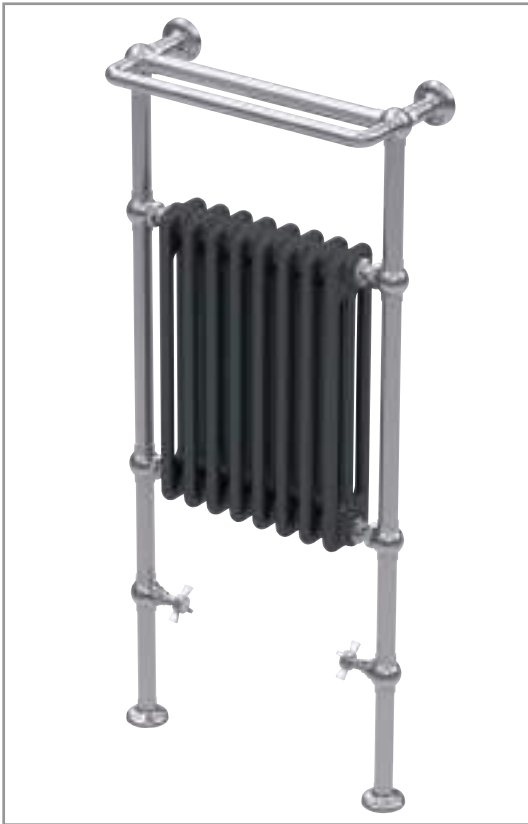
■ SSPVN3/1CR • Radiatore a pavimento con inserto in ghisa e barra porta salviette mm.1185x545 DT60° Kcal/h 653,6 - Watt 758 Radiateur de sol avec insert en fonte et barre porte serviette 1185x545mm. DT60° Kcal/h 653,6 - Watt 758 Floor mounted radiator with cast iron insert and towel rail 1185x545mm. DT60° Kcal/h 653,6 - Watt 758
